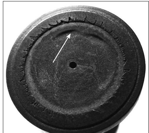
Picture 2: Cavitation of the piston shoes. All pistons must be replaced within the next 500-1,000 hours.
